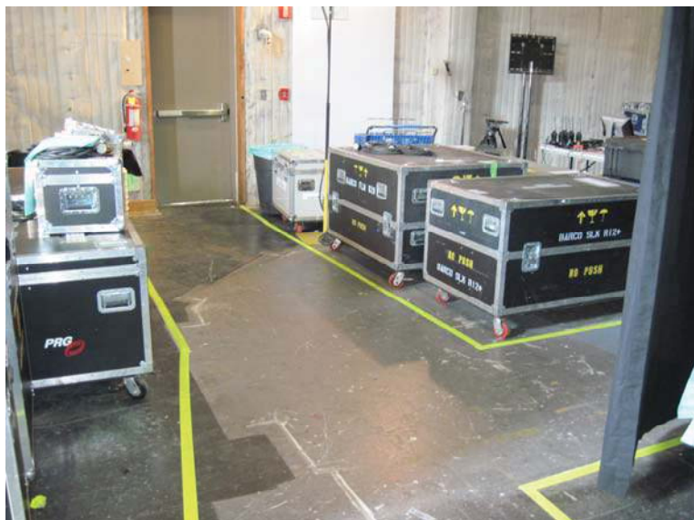
Fig. 4-1 – Marked fire aisle to door. When loading, moving and storing equipment and equipment containers, it is easy to forget that an aisle must remain open for egress. Marking the aisle with bright tape helps remind everyone that an aisle must be maintained to allow for access to the exit. Keeping the marked area completely clear is an important part of an effective safety culture.
