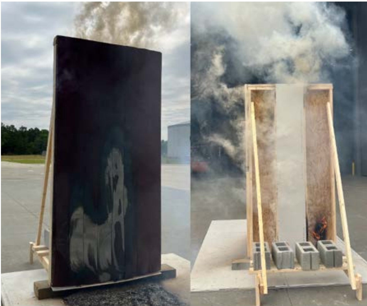
Figure 4. a. Typical exterior wall assemblies constructed on the exterior with noncombustible metal siding. Photo courtesy by Milad Shabaniyan, IBHS.
