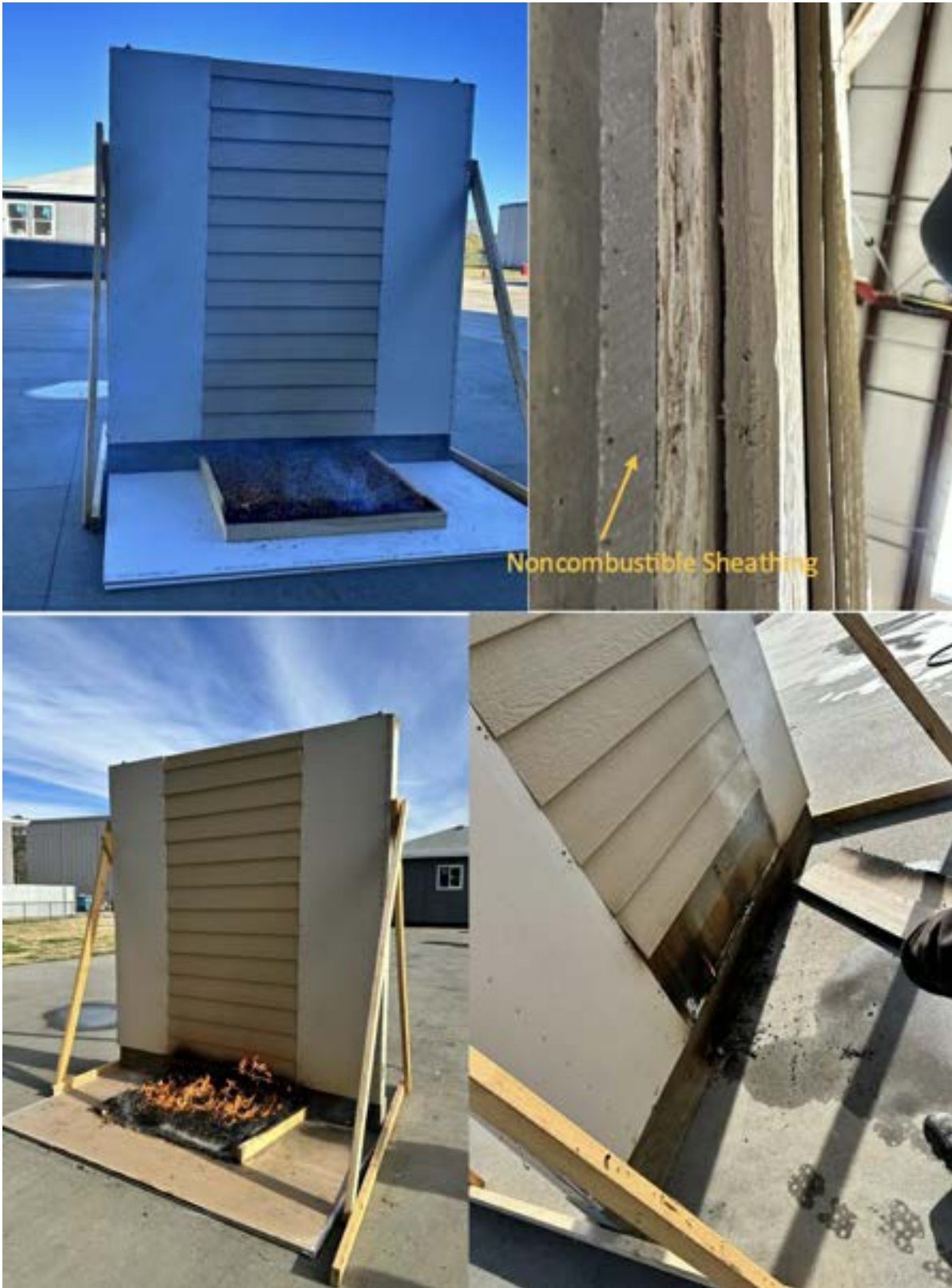
Figure 3. b. 1-hr FRR assembly with noncombustible sheathing material. Photo courtesy by Milad Shabanian, IBHS.
