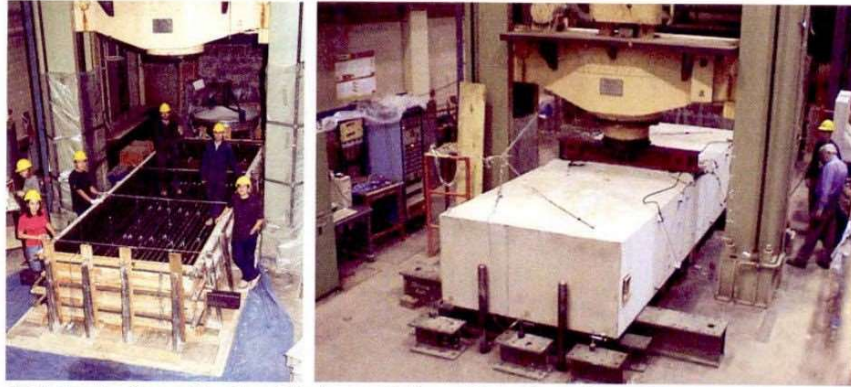
Fig. 8: Construction and loading of the large, wide beam, AT-1 under testing machine at the University of Toronto
