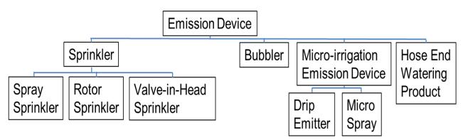
EMISSION DEVICE. An irrigation system component that is used to dispense irrigation water to the landscape at a specific rate.
