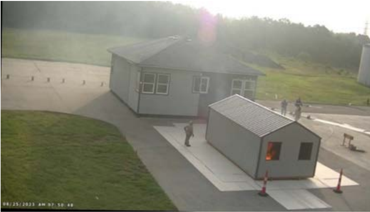
Figure 1. a. The test setup for wind driven building to building fire spread tests. The target building has an hour fire resistant rated wall assembly.
