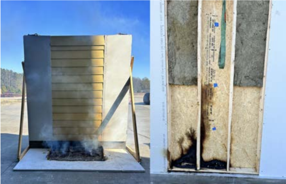
Figure 4. b. Typical exterior wall assemblies constructed on the exterior with noncombustible fiber cement siding material. Photo courtesy by Milad Shabaniyan, IBHS.
