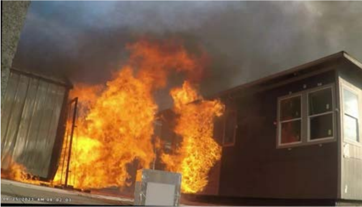
Figure 1. c. fire spread on the surface and flames touching all components in about 10 seconds on left side.
