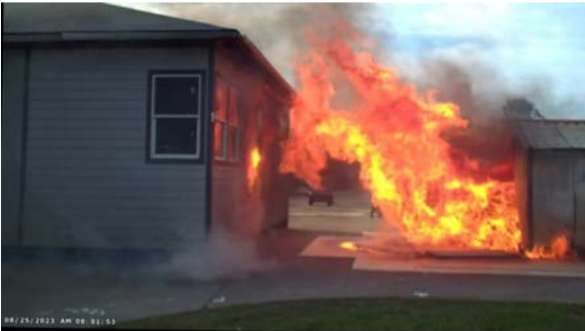
Figure 1. a. The test setup for wind driven building to building fire spread tests. The target building has an hour fire resistant rated wall assembly.
