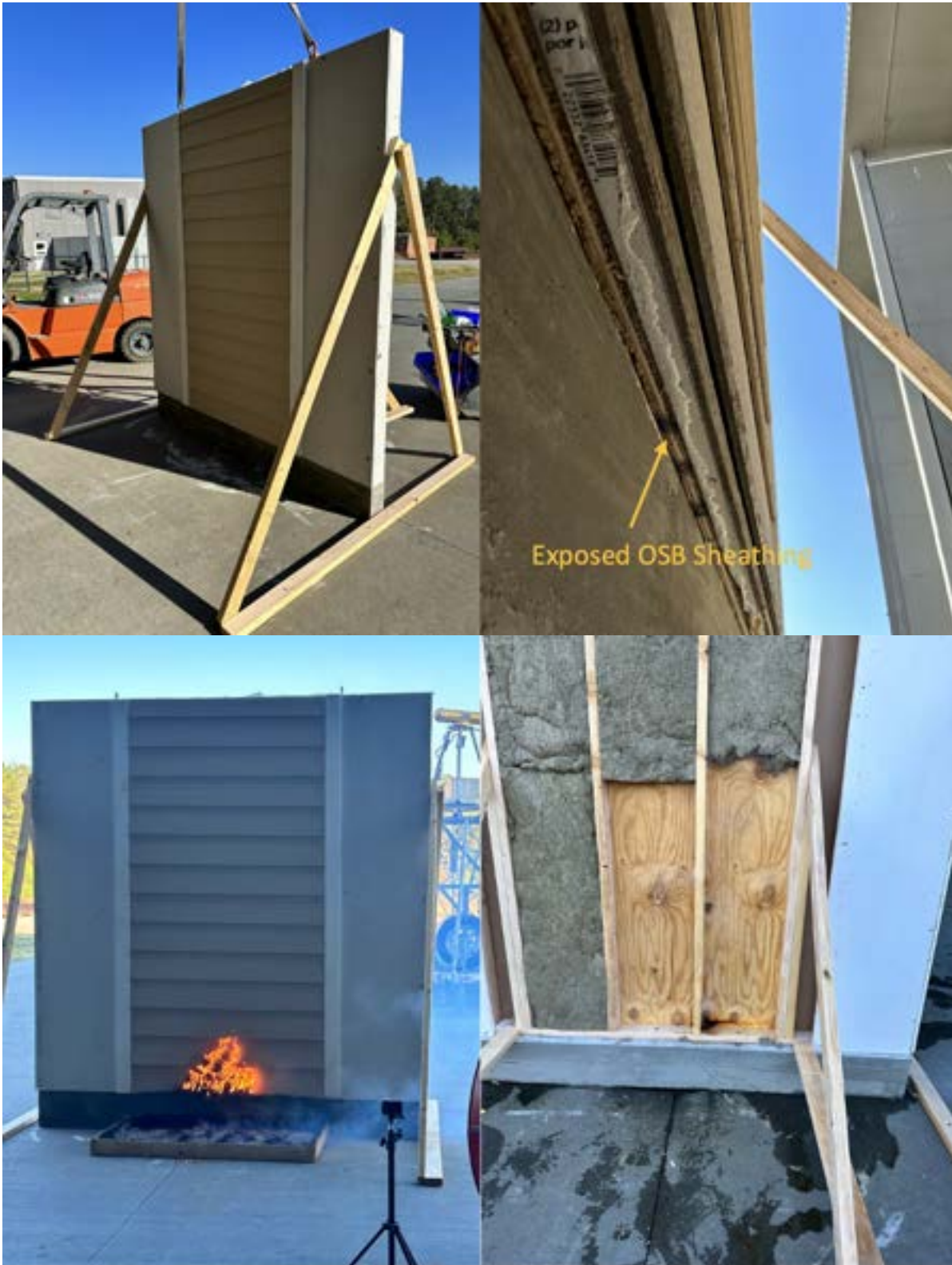
Figure 3. a. 1-hr FRR assembly with unprotected OSB Sheathing material at the bas3. Photo courtesy by Milad Shabani, IBHS.
