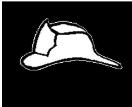
FIGURE 3007.8 FIRE SERVICE ACCESS ELEVATOR SYMBOL
