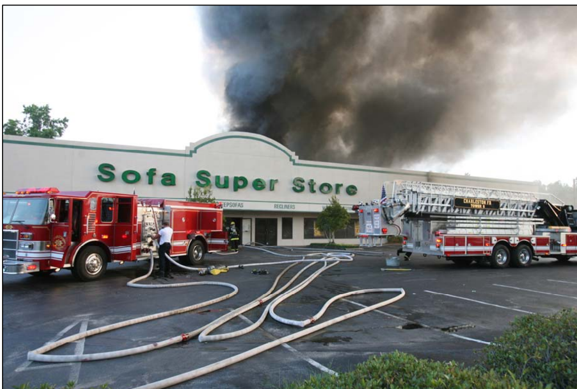
Photo 12: The scene at the front of the store at 19:31:23. Note the lack of pressure evidenced by the kinks in the supply line feeding Engine 11. (Photo courtesy Charleston Post and Courier)
