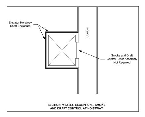
**713.14 Elevator, dumbwaiter and other hoistways.** Elevator, dumbwaiter and other hoistway enclosures shall be constructed in accordance with Section 713 and Chapter 30.
