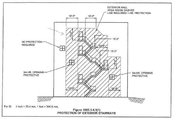
So, if the walls on each side of the stair have to be protected, how can a large opening where the door occurs be removed and have an unprotected connection to the interior corridor.
