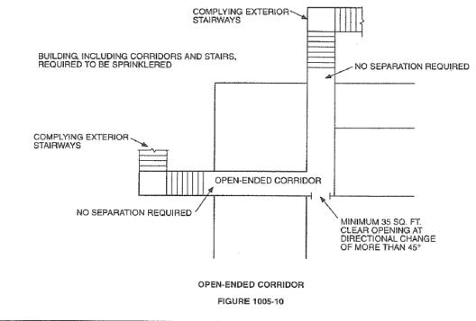
Here is the original code change that inserted the provision. Notice the statement "The purpose of this analysis was to determine if an equivalent level of life safety could be achieved by the design of an open breezeway in comparison to an enclosed corridor or balcony for these multifamily buildings."
