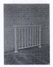
Test Barrier 4B – Barrier to a height of 1000mm height- Standard Slimline Eclipse 'Tekapo' Balustrade system with vertical tube infill (with no opening exceeding 100mm) from a height of 100mm from ground to handrail height of 1000mm.
