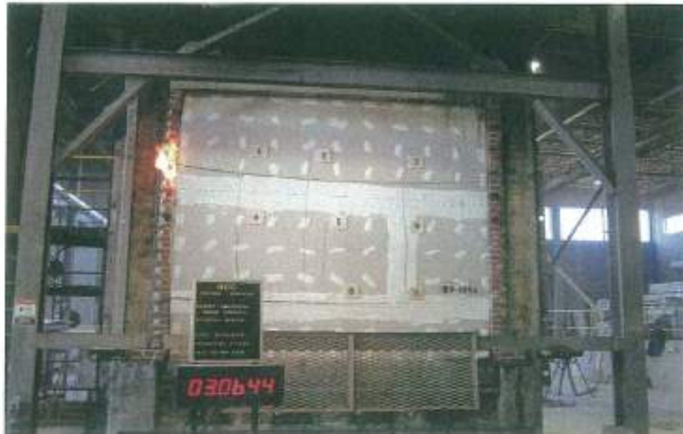
Unexposed Side – Increased Flaming at Wall Assembly Perimeter
