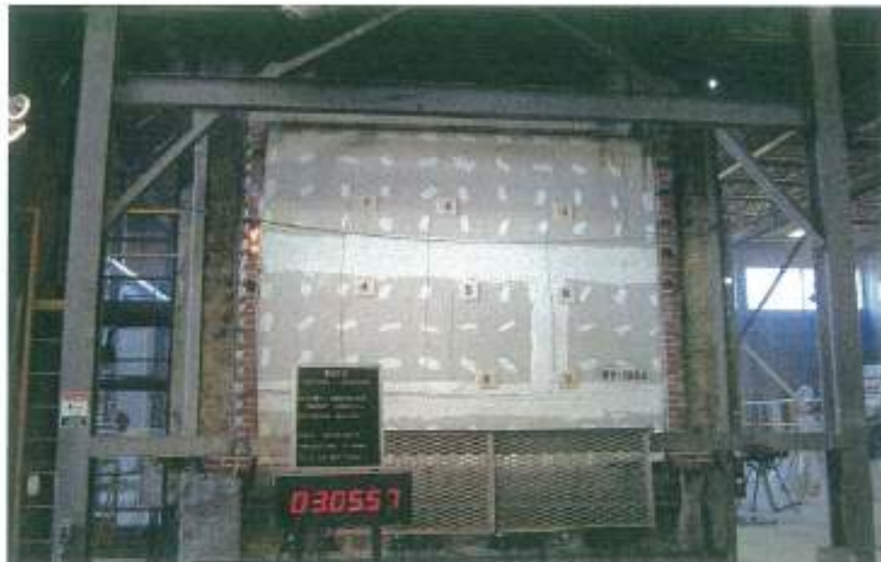
Unexposed Side – Flaming at Wall Assembly Perimeter
