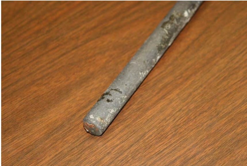
Figure 7. ASTM E119 Furnace Temperature Probe.
